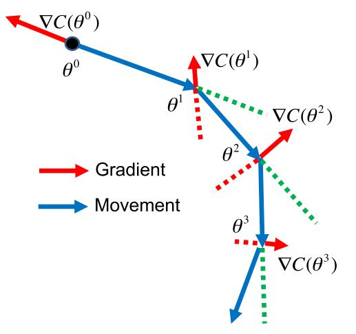
Start at position  $\theta^0$ Momentum  $v^0 = 0$ Compute gradient at  $\theta^0$ Momentum  $v^1 = \lambda v^0 - \eta \nabla C(\theta^0)$ Move to  $\theta^1 = \theta^0 + v^1$ Compute gradient at  $\theta^1$ Momentum  $v^2 = \lambda v^1 - \eta \nabla C(\theta^1)$ Move to  $\theta^2 = \theta^1 + v^2$
